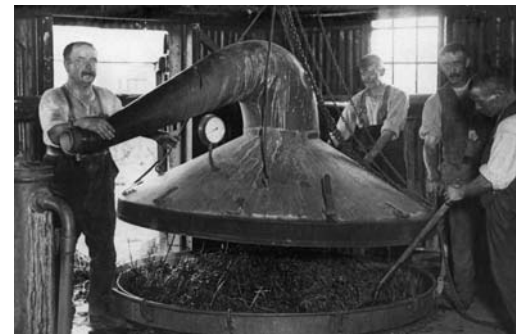
Preparing the retort for distilling mint at Miller's works, Hackbridge
